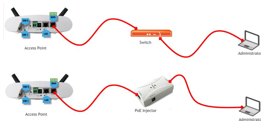
4. Factory default the AP by holding in the reset button for 10 seconds. This will reset the APs IP address to 192.168.0.1.
